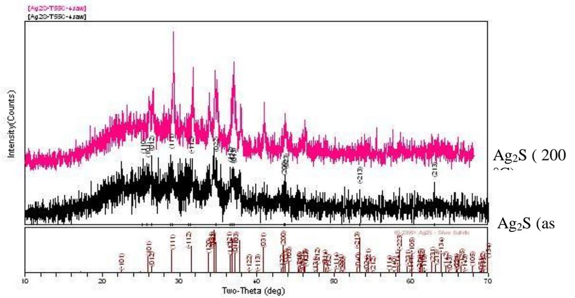
Fig 6.1 XRD patterns recorded for as prepared  $\text{Ag}_2\text{S}$  thin films on glass substrate and after heating in air at 200 °C for 3h
