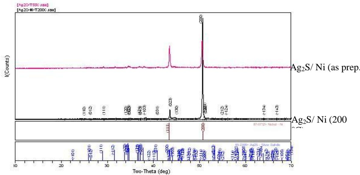
Fig 6.2 XRD patterns for an  $\text{Ag}_2\text{S}$  films deposited on Ni substrate and heated in air at 200°C for 3h
