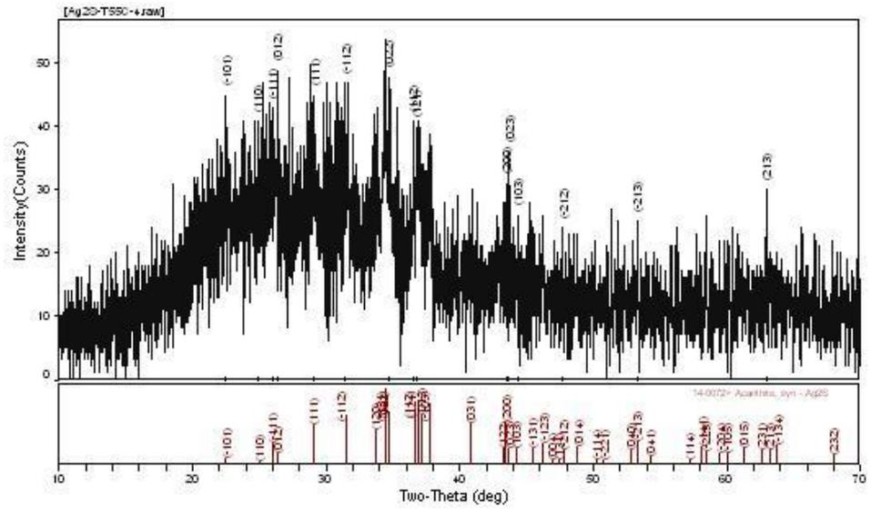
Fig 3.1 XRD pattern recorded for as prepared Ag<sub>2</sub>S thin films on glass substrate
