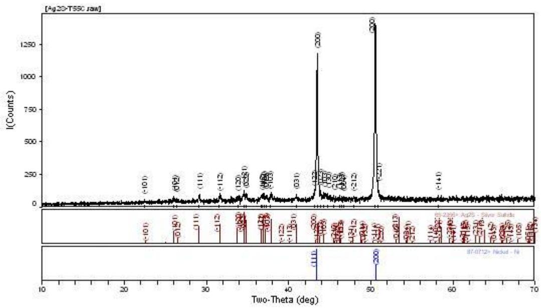
Fig 3.3 XRD pattern of as prepared Ag<sub>2</sub>S/ Ni thin films
