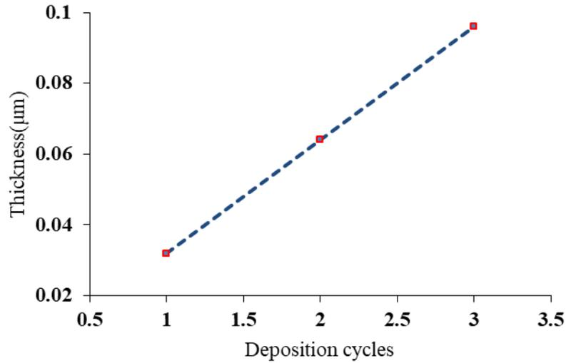
Fig 6.4 Plot of film thickness vs. deposition cycles for Ag<sub>2</sub>S films
