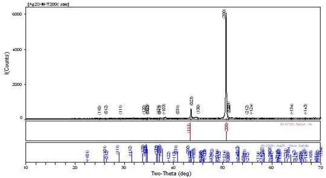
Fig 3.4 XRD pattern recorded for annealed  $\text{Ag}_2\text{S}/\text{Ni}$  thin films in air at  $200^\circ\text{C}$  for 3 h
