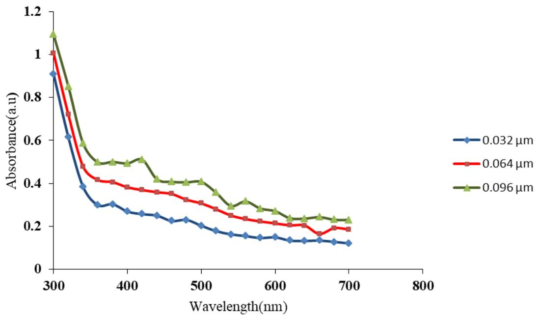
Fig 4.6 Plots of absorbance spectra of selected samples of  $\text{Ag}_2\text{S}$  thin films
