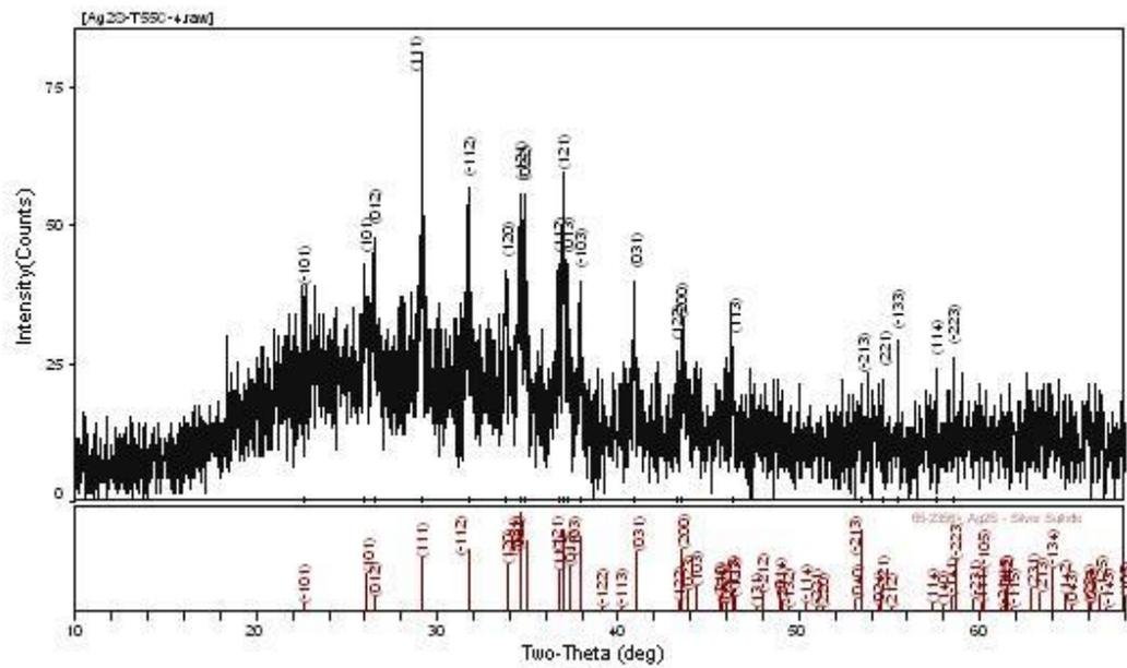
Fig 3.2 XRD pattern of Ag<sub>2</sub>S thin films on glass substrate after annealing in air at 200°C for 3 h
