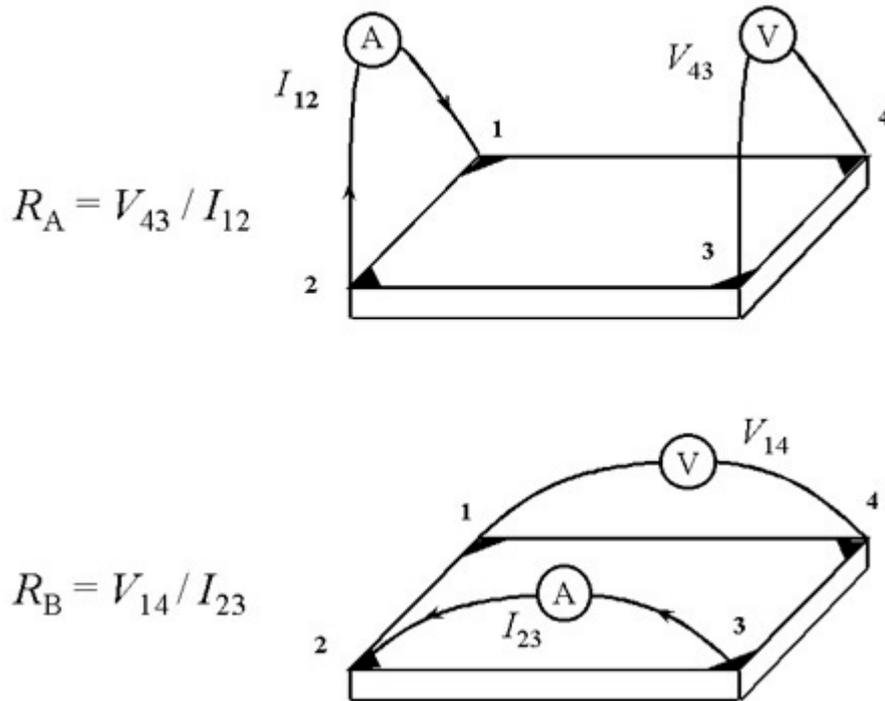
Fig 5.3 Schematic of a Van der Pauw configuration used in the determination of the two characteristic resistances  $R_A$  and  $R_B$
