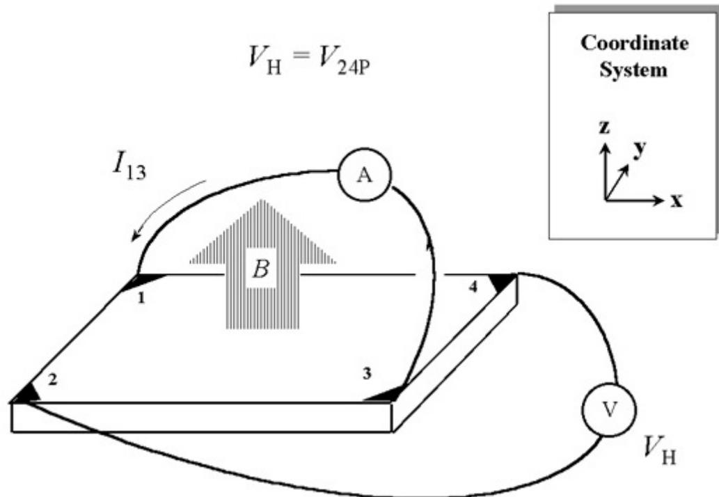
Fig 5.4 Schematic of a Van der Pauw configuration used in the determination of the Hall voltage  $V_H$ .
