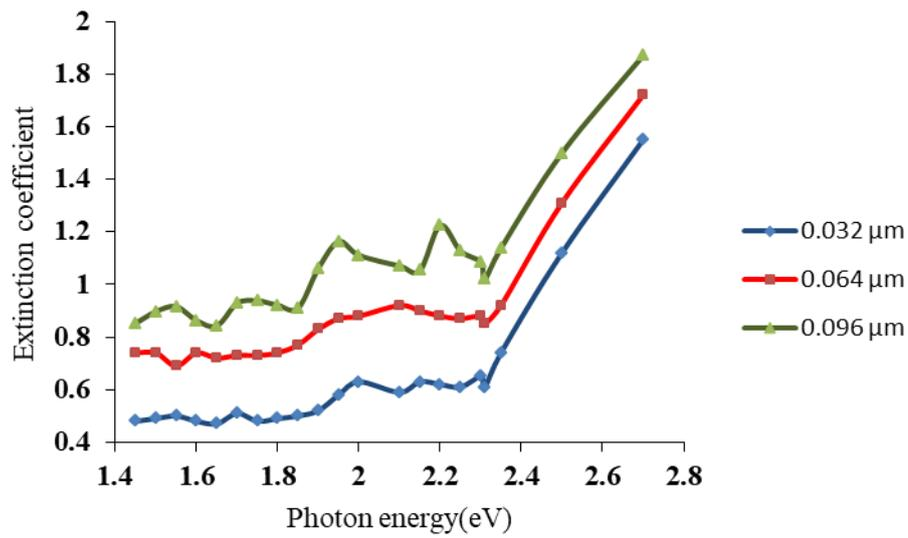
Fig 4.9 Extinction coefficient ( $k$ ) versus photon energy ( $h\nu$ ) for  $\text{Ag}_2\text{S}$  thin films with different thickness
