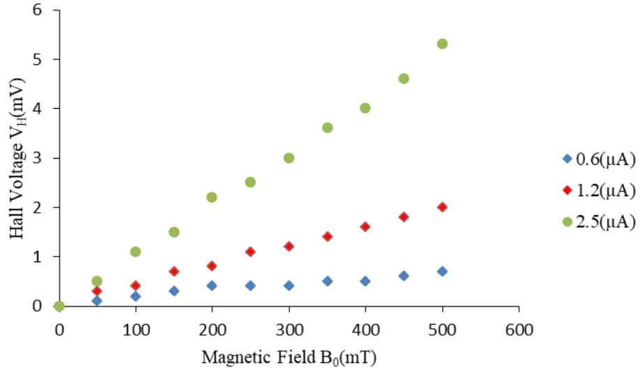
Fig 5.8 Variation of Hall voltages with Magnetic field
