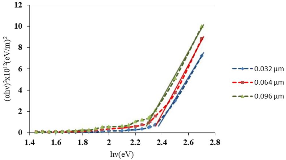
Fig 4.7 Variation in  $(\alpha h\nu)^2$  with photon energy ( $h\nu$ ) for  $\text{Ag}_2\text{S}$  films in different thickness
