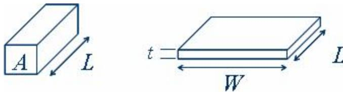
Fig 5.5 Geometry for defining resistivity (left) and sheet resistance (right)
